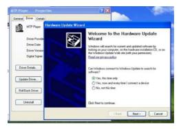
Step 5: Follow the tips of Dialog Box by clicking the "Next >" button to finish updating. The procedure should be : Install from a list or specific location (Advanced) – Don't search. I will choose the driver to install – USB Mass Storage Device – Finish. The Removable Disk will appear in My Computer.
